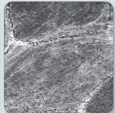
PeakForce QNM topography image (left) and corresponding modulus image (right) of living MDCK cells. Cell structures corresponding to actin fibers show higher modulus (lighter) while cell surface features, believed to be microvilli, appear softer (darker) than the cell membrane itself. (1 kHz PeakForce QNM, 32 \mu m image).
