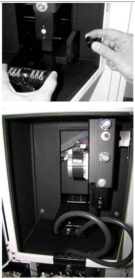
The picture above shows the view from inside when the tubing is fitted.
